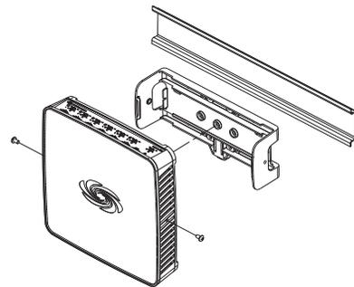
**NOTE:** Do not use the supplied screws to mount the bracket to the bottom of the MMX-6-USB if the device will be mounted on a DIN rail. Removing the MMX-6-USB from the DIN rail is not possible.
