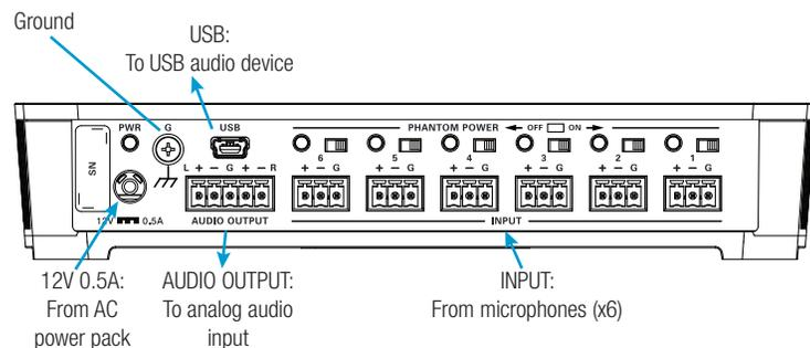
**NOTE:** The AUDIO OUTPUT and USB ports can be connected simultaneously.
